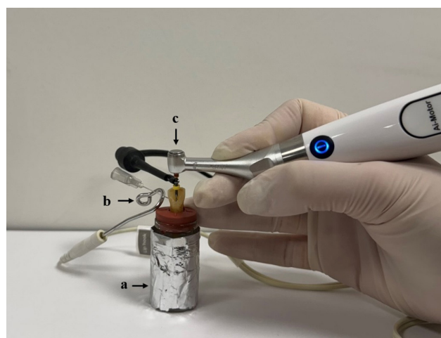
Figure 1. Experimental apparatus used to evaluate apically extruded debris. (a) The cover of the outer surface of a glass tube with aluminum foil. (b) The placement of the lip clip on the syringe in order to complete the circuit. (c) The operation of the file.
